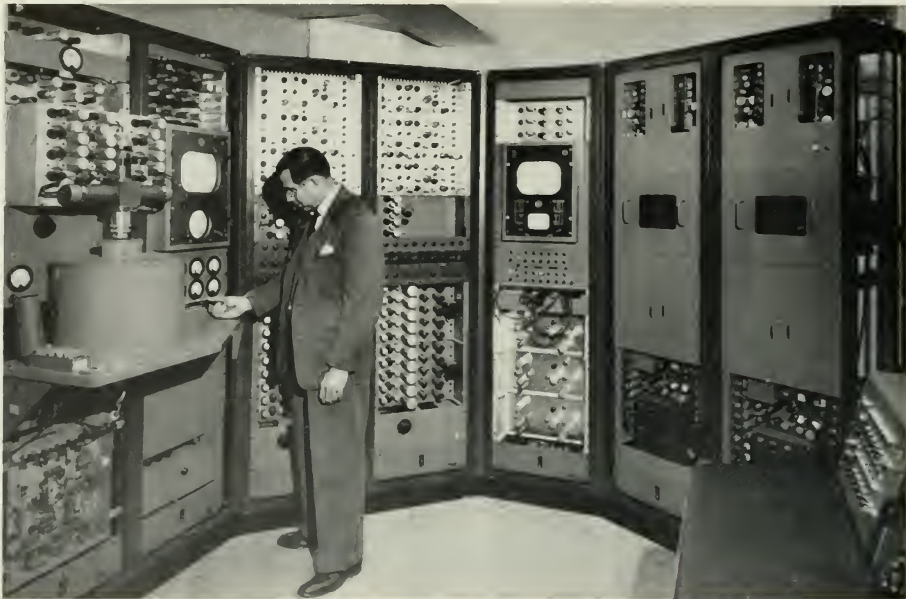
STUDIO CONTROL UNITS OF NEW RCA ALL-ELECTRONIC, HIGH-DEFINITION COMPATIBLE COLOR TELEVISION SYSTEM AS INSTALLED AT NBC STATION WNBW IN WASHINGTON. RAY D. KELL, HEAD OF THE TELEVISION SECTION, RCA LABORATORIES, IS OPERATING THE MONOCHROME MONITOR.
